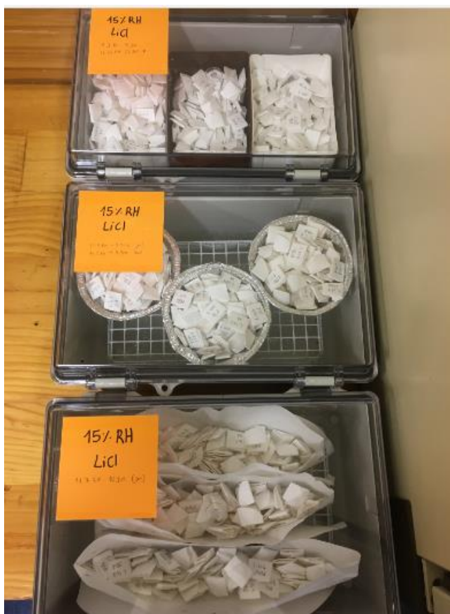
Appendix Q. Seeds envelopes reaching the RH equilibrium in boxes containing the LiCl solutions at 20 °C.
