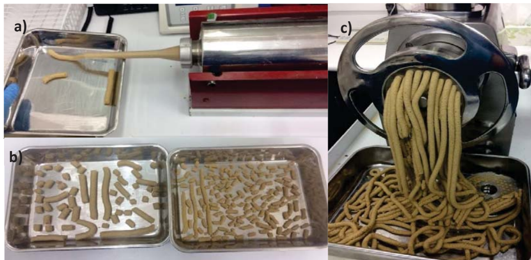
Figure 3-4 a) Sausage maker b) Sausage pellets left tray and mincer pellets right tray c) Mincer with 8mm pierced disk on
