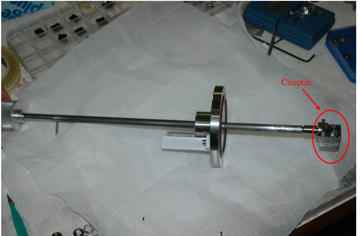
Figure 1.2: The coupon holder with the coupon fixed on it using a carbon tape.
