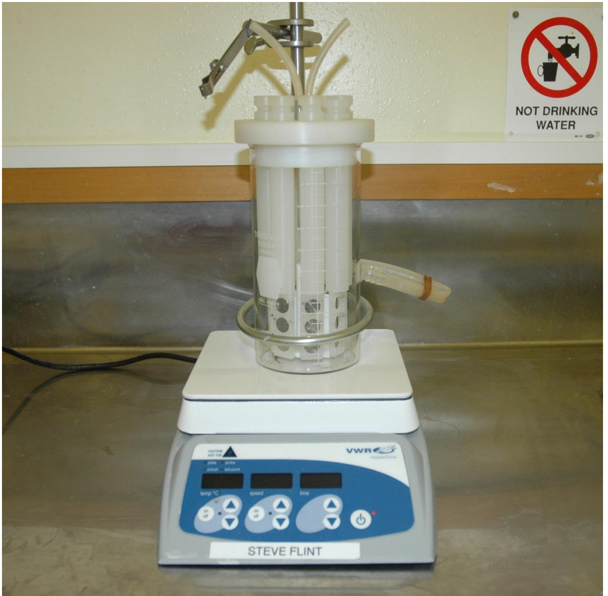
Figure 1.3: CDC biofilm reactor used for the experiments in the study.
