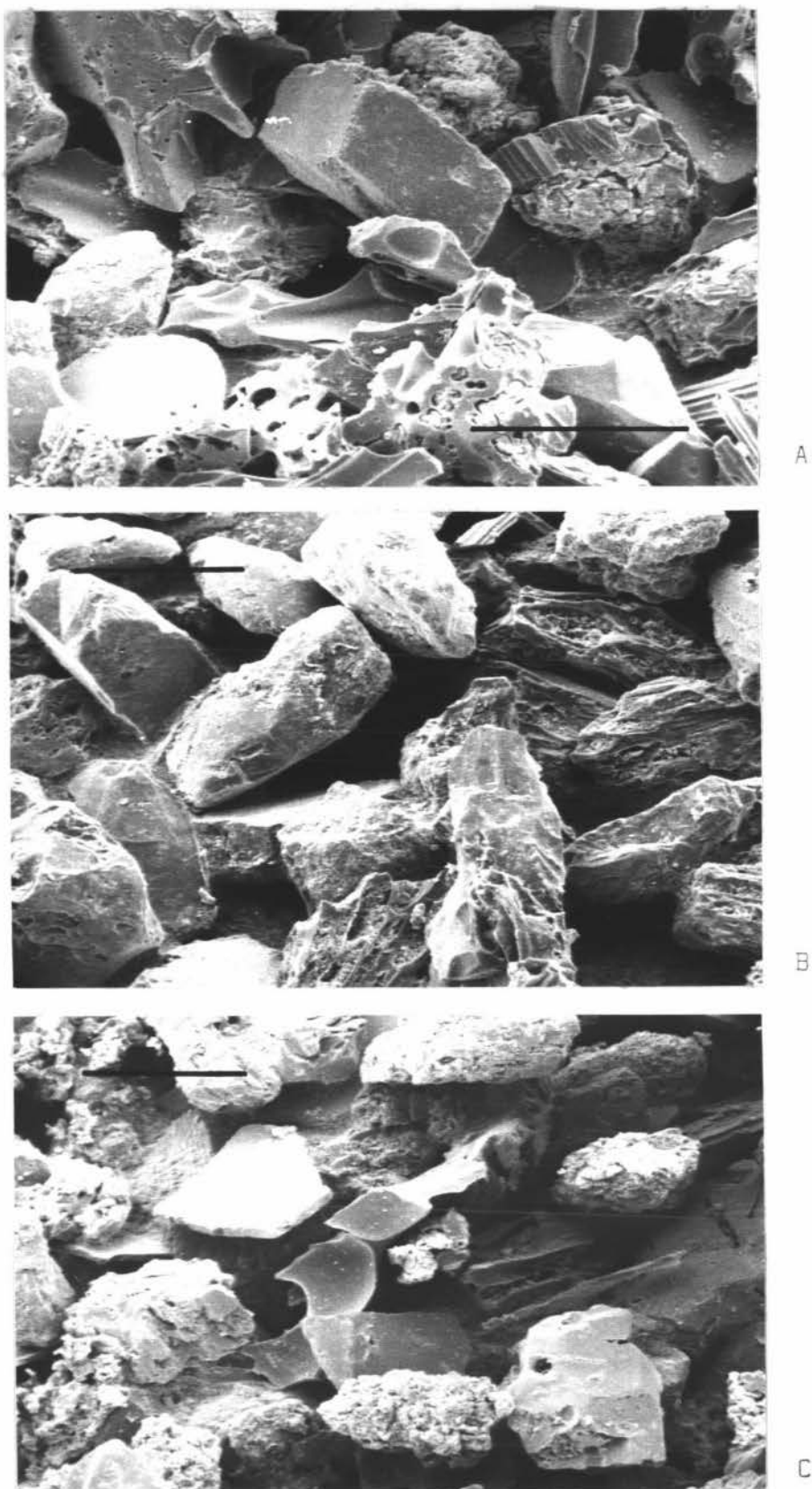
FIGURE 17: Scanning electron micrographs of Post-Okareka loess particles from sections: A - close ( AL_1 ), B - intermediate ( CL_2 ) and C - furthest ( EL_1 ) to ash source (Bars = 200\mu m ). With increasing distance from ash source, grain angularity decreases and the proportion of silt-size aggregates increases.
