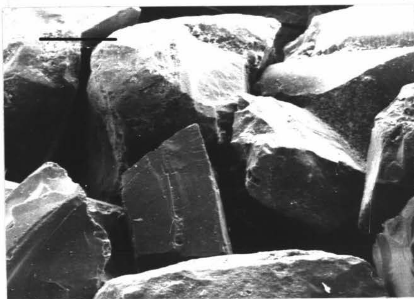
FIGURE 7A: Scanning electron micrograph of quartz grains separated from Okareka Ash samples (Bar = 200 \mu m).
