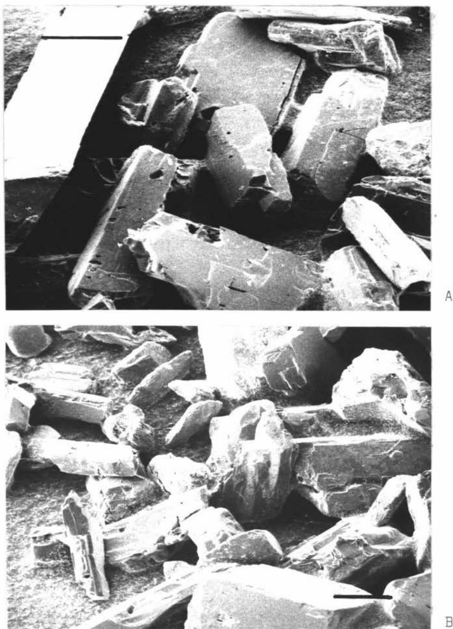
FIGURE 9: Scanning electron micrographs of hornblende grains separated from: A - Okareka Ash (Bar = 200 \mu m) B - Post-Okareka loess (Bar = 250 \mu m) Grains in both SEM's show only minimal evidence of weathering.
