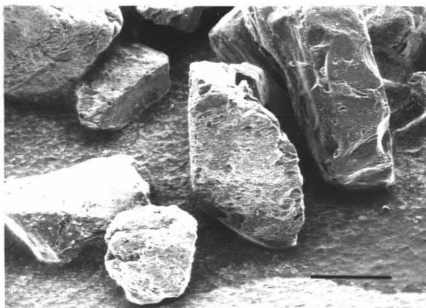
FIGURE 13: Scanning electron micrograph of plagioclase feldspar grains separated from Post-Okareka loess samples (Bar = 500 \mu m).
