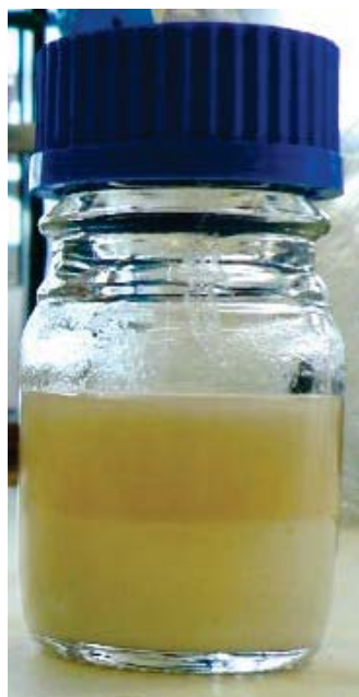
Figure 16. Image of a loaded hydrogel illustrating the separation effect. Hydrogel composition: 9 g sodium salicylate, 1.0 g alginate, 1.0 g calcium chloride, and 60 mL water.
