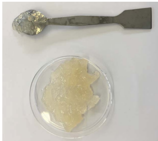
Figure 15. Image of hydrogel B4 and its ability to coat the back of a spoon. Hydrogel composition: 1.0 g alginate, 20 mL water, and 0.2 g calcium chloride.
