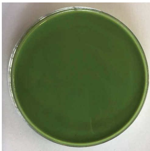
Figure 18. Image illustrating the formation of copper salicylate during the preparation of a hydrogel. Hydrogel composition: 9 g sodium salicylate, 1.0 g alginate, 1.0 g copper sulfate, and 60 mL water
