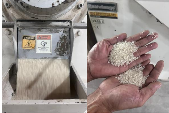
Figure 12: Grading after polishing at CDo factory
