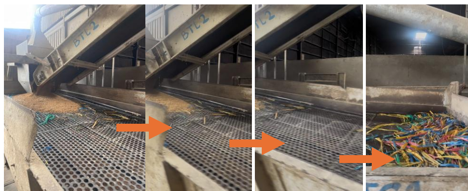
Figure 3: Screening in CDo factory
