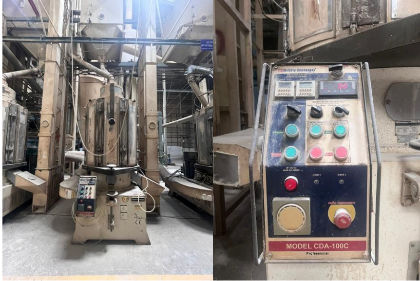
Figure 9: Whitener and its control panel
