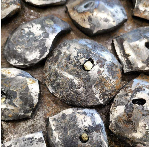
Figure 43. Pierced, filled with brass and surface ground, Massey University Design workshop, Te Whanganui-a-Tara, 2025.
