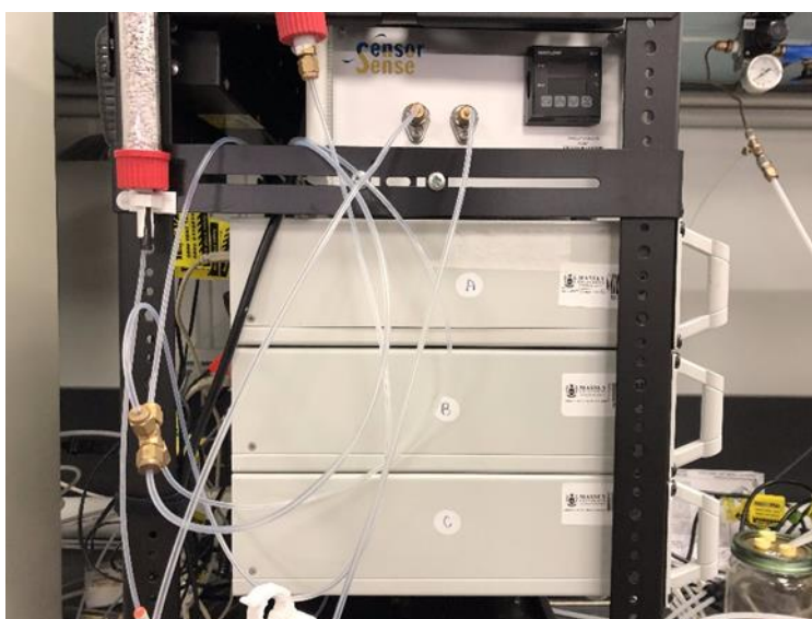
Figure 5.3 ETD-300 was used to measure the ethylene concentration
