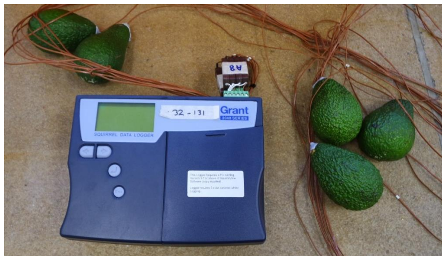
Figure 3.3 Thermocouples connected to data loggers using for seed surface temperature measurement
