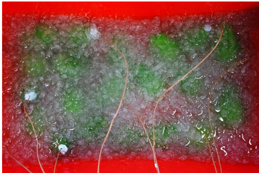
Figure 3.2 Avocado fruit were immersed in ice water during CST at 0 °C for 2 h with the thermocouple used for seed surface of the fruit and water temperature observation
