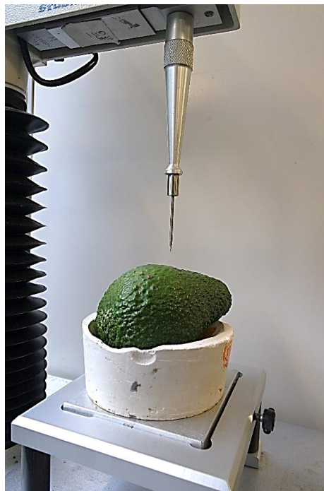
Figure 3.4 Puncture test using TA.XT Plus Texture Analyser with a needle probe
