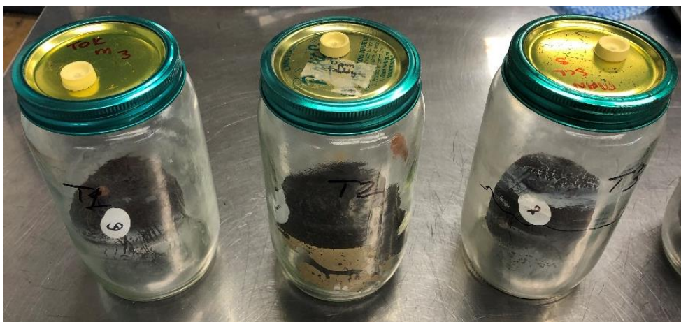
Figure 6.2 Gas samples were taken for respiration rate and ethylene production rate from a set of 10 glass jars which contained one fruit after 15 minutes
