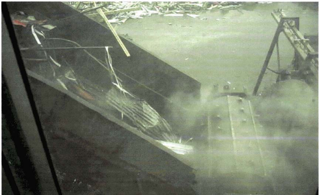
Photograph 8: Metal going down the chute into the shredder
