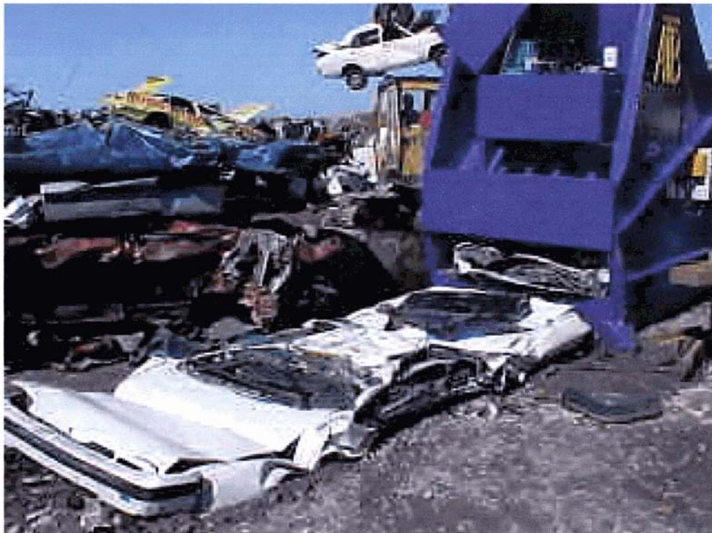
Photograph 4: Car hulk emerging from ELV Flattener
