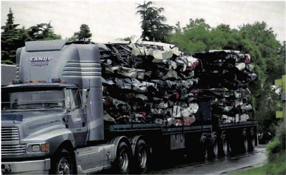
Photograph 5: Crushed car hulks being transported to the Metal Shredder
