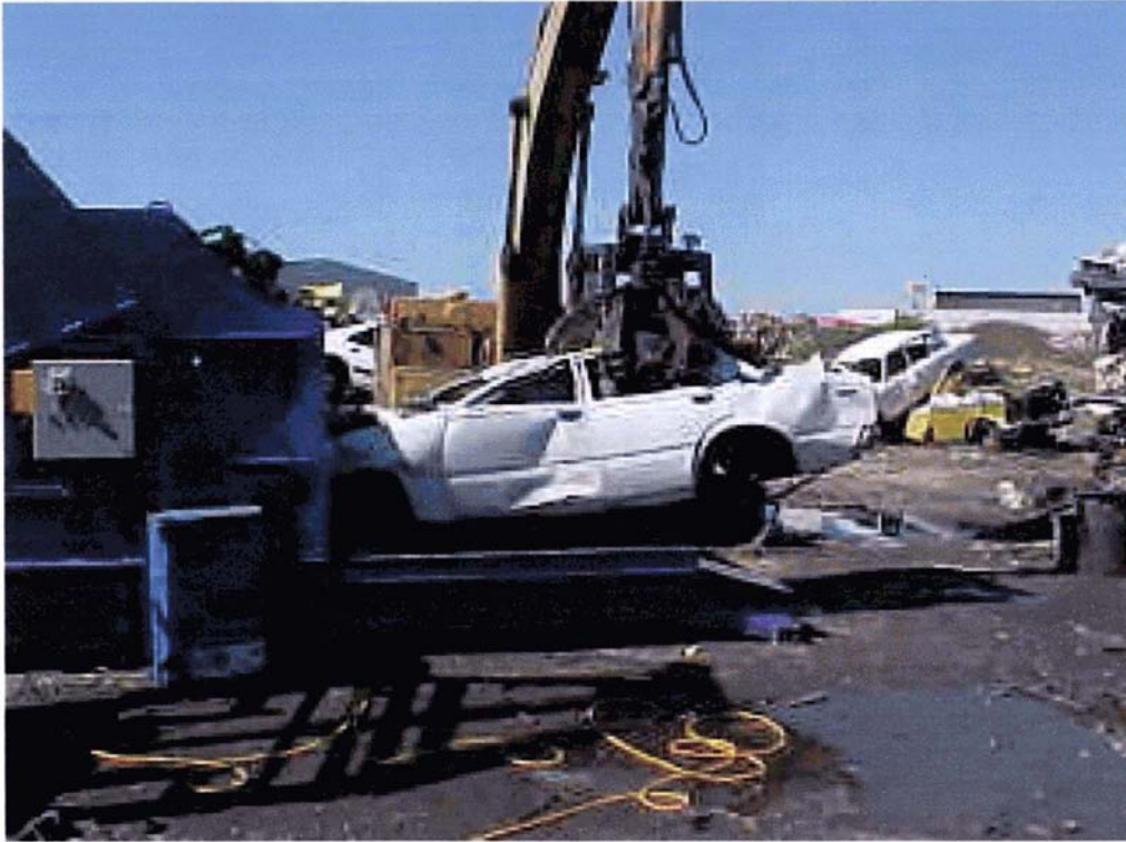
Photograph 3: Car hulk entering ELV Flattener
