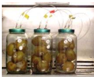
Figure 3-3: Sealed glass jars (with kiwifruit) fitted with two rubber septum to connect tubes to and from the valve controller box of the ethylene detector used in determination of ethylene production.
