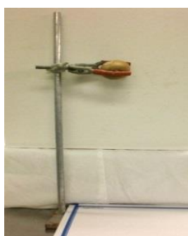
Figure 5-1: Method used to drop kiwifruit from different heights
