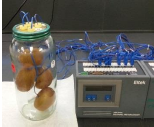
Figure 6-1: Method established to measure internal temperature of kiwifruit by using a Squirrel temperature data logger with thermocouples (SQREM1200, Eltek, Cambridge, United Kingdom).
