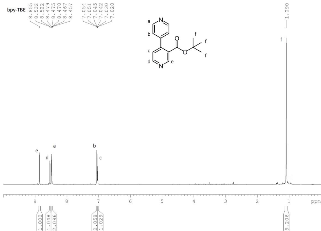
Figure 4.8 ^1\text{H-NMR} spectroscopic analysis of bpy-TBE in \text{CDCl}_3 .
