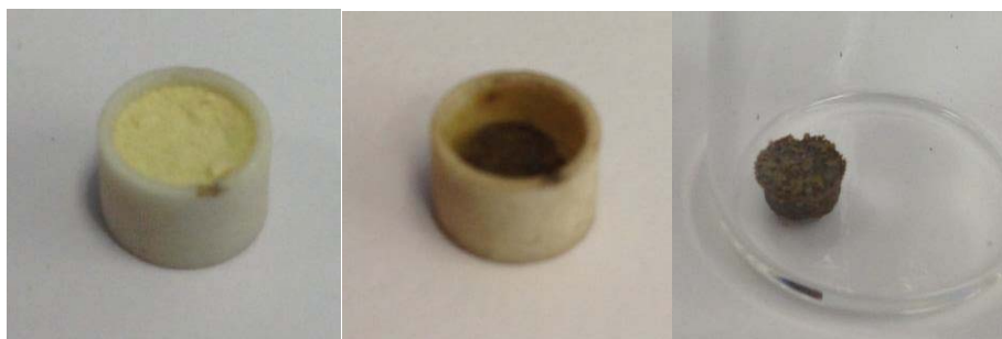
Figure 2.10 Images of 1,4-bdc-NHCOOEt before thermolysis (left), after thermolysis (middle), and cake removed from alumina pan (right).
