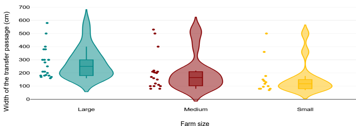
Figure 6. Distribution of different transfer passage widths on small (<180 lactating cows), medium (181 to 899 lactating cows), and large (>900 lactating cows) farms in a cross-sectional study of 62 Iranian dairy farms. The solid line in box shows median, lower end of the box shows first quartile, top end of the box shows the third quartile, and the whiskers show 95% confidence intervals. Dots show the farms. Colour areas show the distribution of the data.
