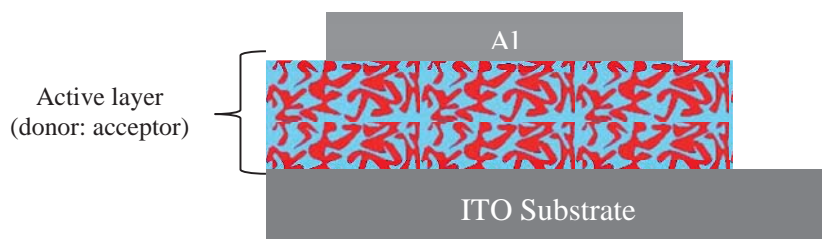
Figure 1.3 Bulk heterojunction solar cell device architecture.
