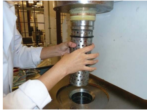
Figure 10: Securing the 2L cylinder by screwing to the upper closure of the pneumatic lifting device.
