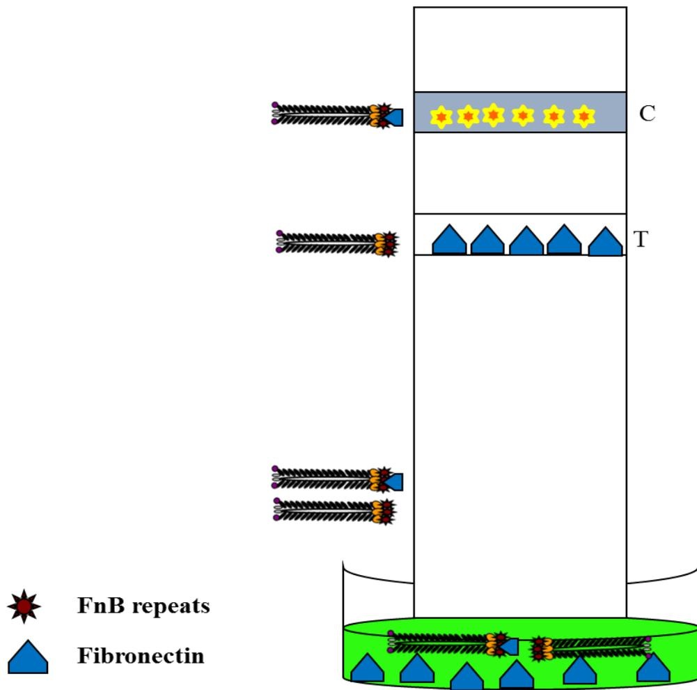
**Figure 4.7 Schematic presentation of dipstick competition assay for quantitative detection of fibronectin using nanophage particles.** All phage particles bound to analyte in the test solution will be retained at ‘C’, the control line, whereas the phage particles that are not bound to fibronectin are retained at test line ‘T’.
