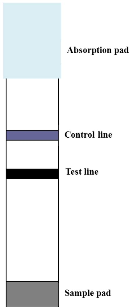
**Figure 2.3 Custom-made dipstick device.** Sample pad which is dipped in sample solution; test strip to capture any analyte bound with detector probe; control or capture strip to capture unbound probe; Absorption pad (cellulose fiber pad to increase volume of analyte absorbed).
