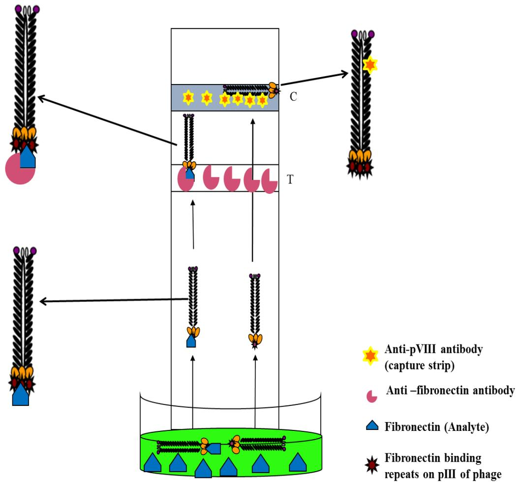
**Figure 4.4 Schematic presentation of dipstick immunoassay developed to test the potential of nanophage particles in diagnostics. C: control line indicating a valid assay; T: test line indicating a positive assay.**
