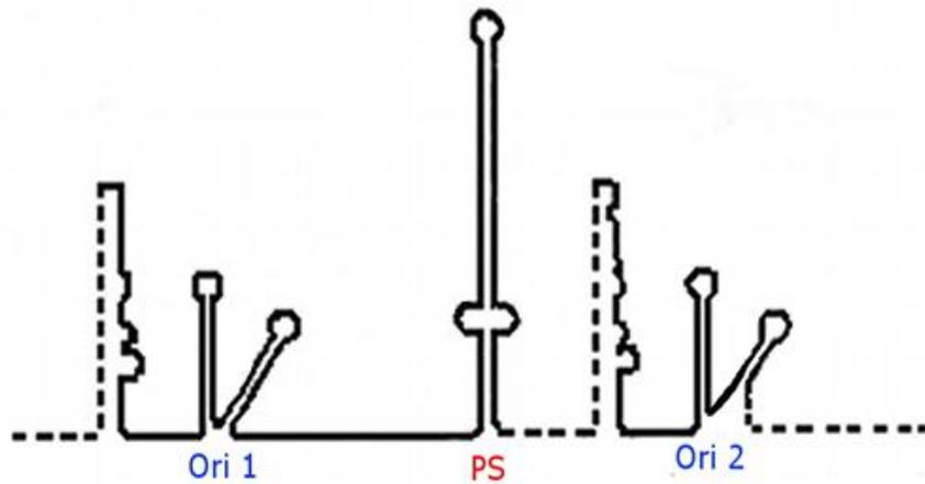
**Figure 1.7 Engineered origin of replication for microphage (nanophage) production.** *Ori1*; wild type positive origin of replication capable initiating as well as terminating rolling circle mode of ssDNA replication. PS; packaging signal, *Ori2*; mutated positive origin of replication acting as terminator only. Figure adapted from (Specthrie et al., 1992) with permission.
