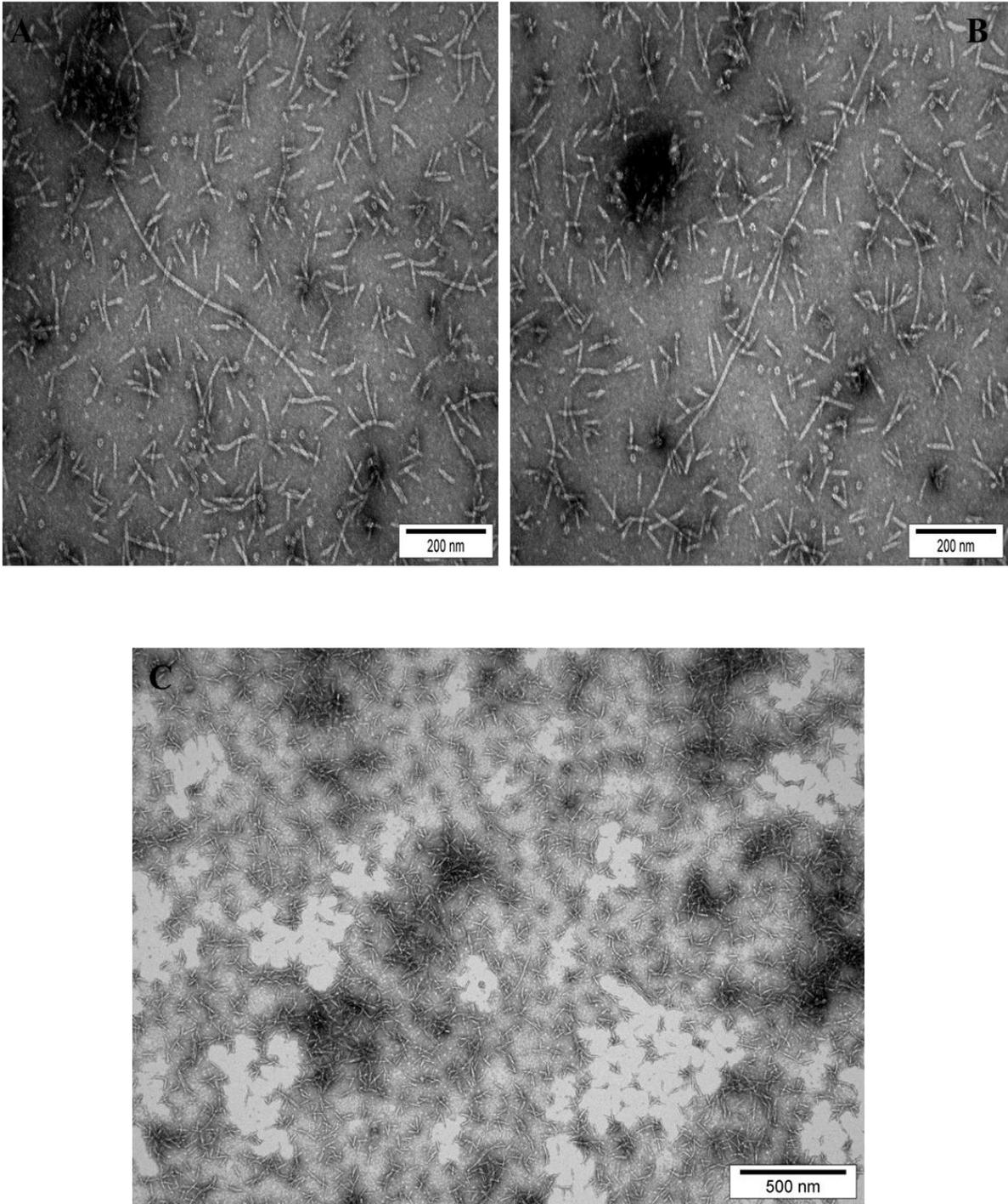
**Figure 6.1 Transmission Electron Micrographs (TEM) of purified nanophage sample EPN1.** The samples were negatively stained using Uranyl acetate. Bar corresponds to 200nm (A & B) and 500nm (C).
