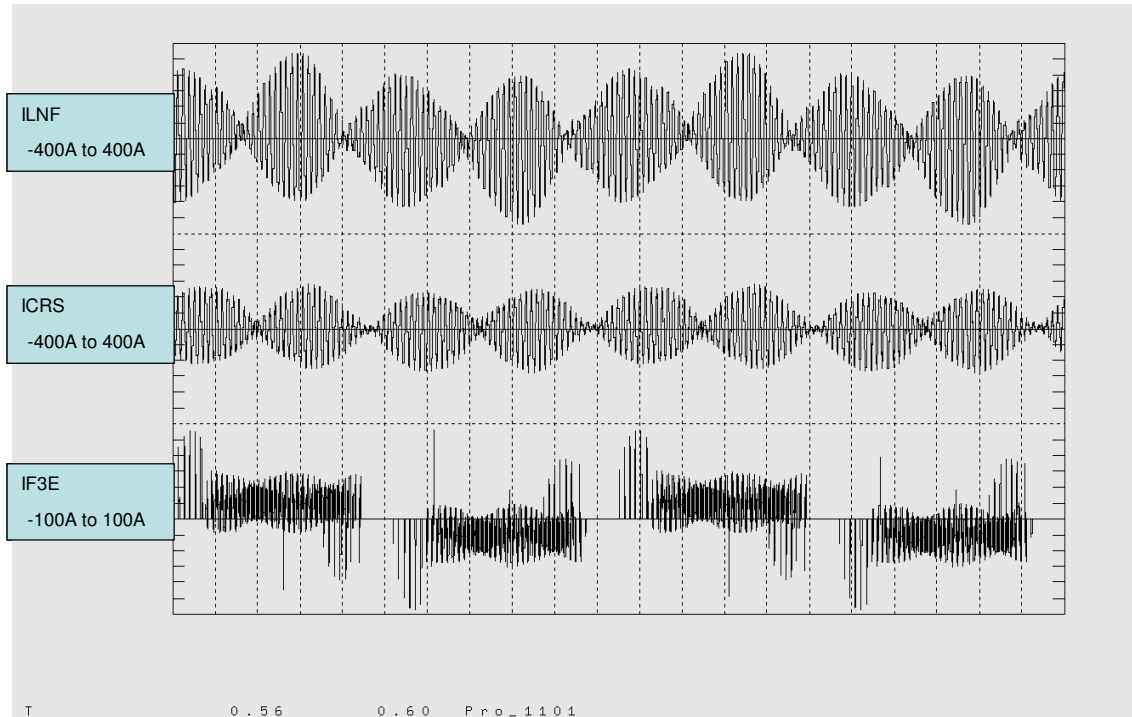
Fig. 5.29: Shape of the F3E currents at an R_{sc} = 96
