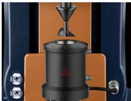
Figure 3.7: Discovery HR-3 hybrid rheometer with a starch pasting cell (TA Instruments, 2018).
