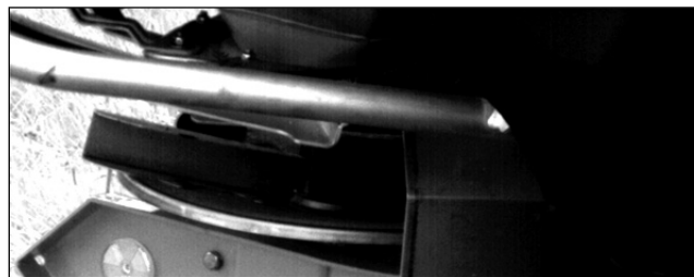
Figure 2. Short vane spinner of the Kuhn Axis 0.215 m spreading Nitrophoska 12-10-10 at 1083 rpm, a still photograph from high speed photometry.
