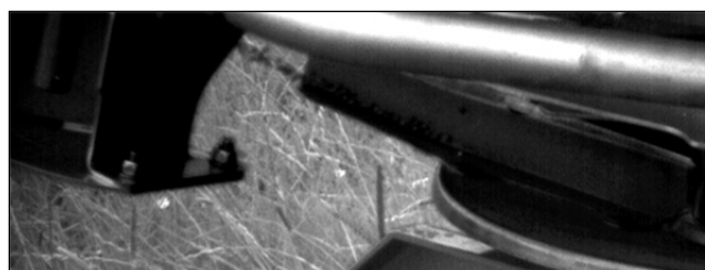
Figure 1. Long vane spinner of the Kuhn Axis 0.285 m spreading Nitrophoska 12-10-10 at 1083 rpm, a still photograph from high speed photometry.
