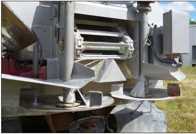
Figure 3. The ACE bin and spreader used to sow SSP.
