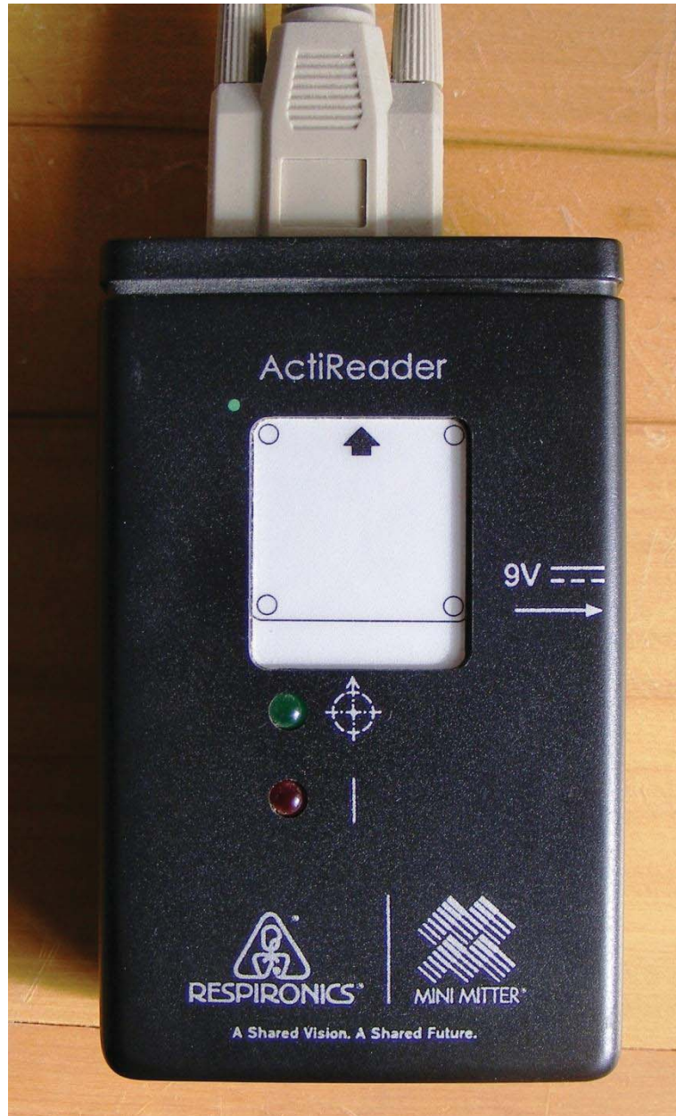
Figure 4.2: ActiReader (MiniMitter, Bend, OR, USA) docking station used to download data from Actical ® activity monitors.
