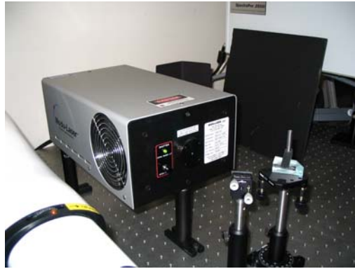
Figure 2.6: The multi-line argon laser and the first Pellin-Broca setup.
