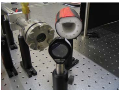
Figure 2.15: The setup of the 532 nm beam dump. SRS light would pass through the dichroic mirror while the 532 nm irradiating light would be reflected into the beam dump.
