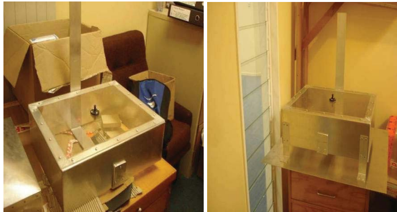
Figure 3-2: Surface gas collectors
