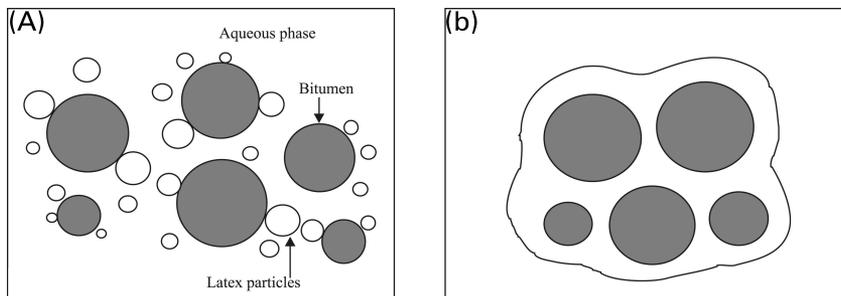
**Fig. 2.** (a) Schematic illustration of the modified emulsion showing the latex particles remaining in the aqueous phase surrounding the bitumen droplets. (b) Evaporation or destabilization of the aqueous phase results in the latex particles forming a continuous polymer film around the bitumen droplets.
