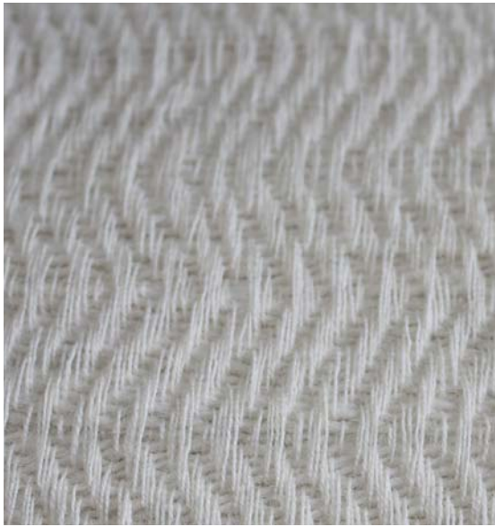
Figure 64. Hard waste yarn, woven using a twill pattern on a straight draft table loom. Author's own (2012)
