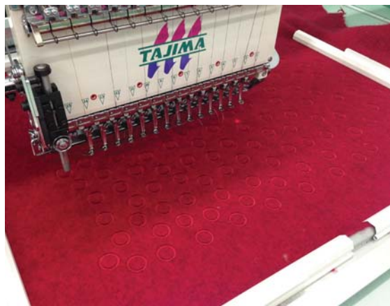
Figure 28. The Digitized design being stitched on the embroidery machine. Author's own (2012)
