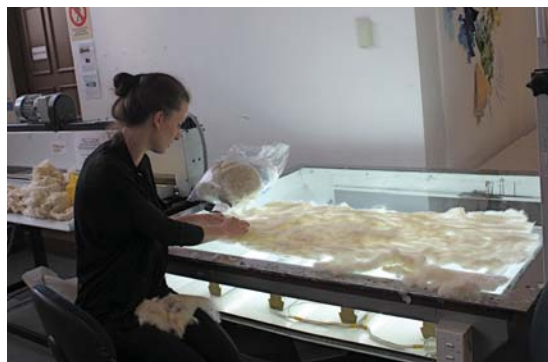
Figure 10. Laying the fleece into fine layers to be needle felted on the felt loom. Author's own (2012)
