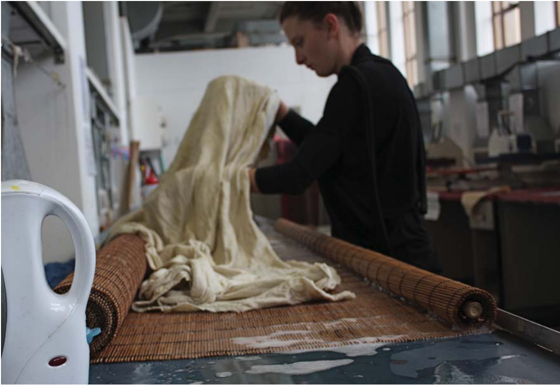
Figure 16. The final stage of the wet felting process, working, fulling the fabric. Author's own (2012)
