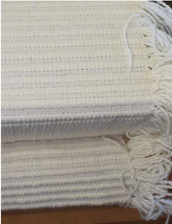
Figure 66. Close up of carpet yarn ribbed sample in progress on the table loom.
