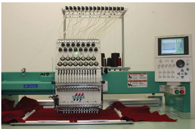
Figure 22. The TAJIMA automatic digital single head embroidery machine, TFMX series, Author's own (2012)
