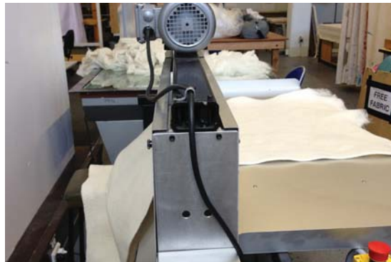
Figure 13. Final stages of the felt being fed through the loom. Author's own (2012)
