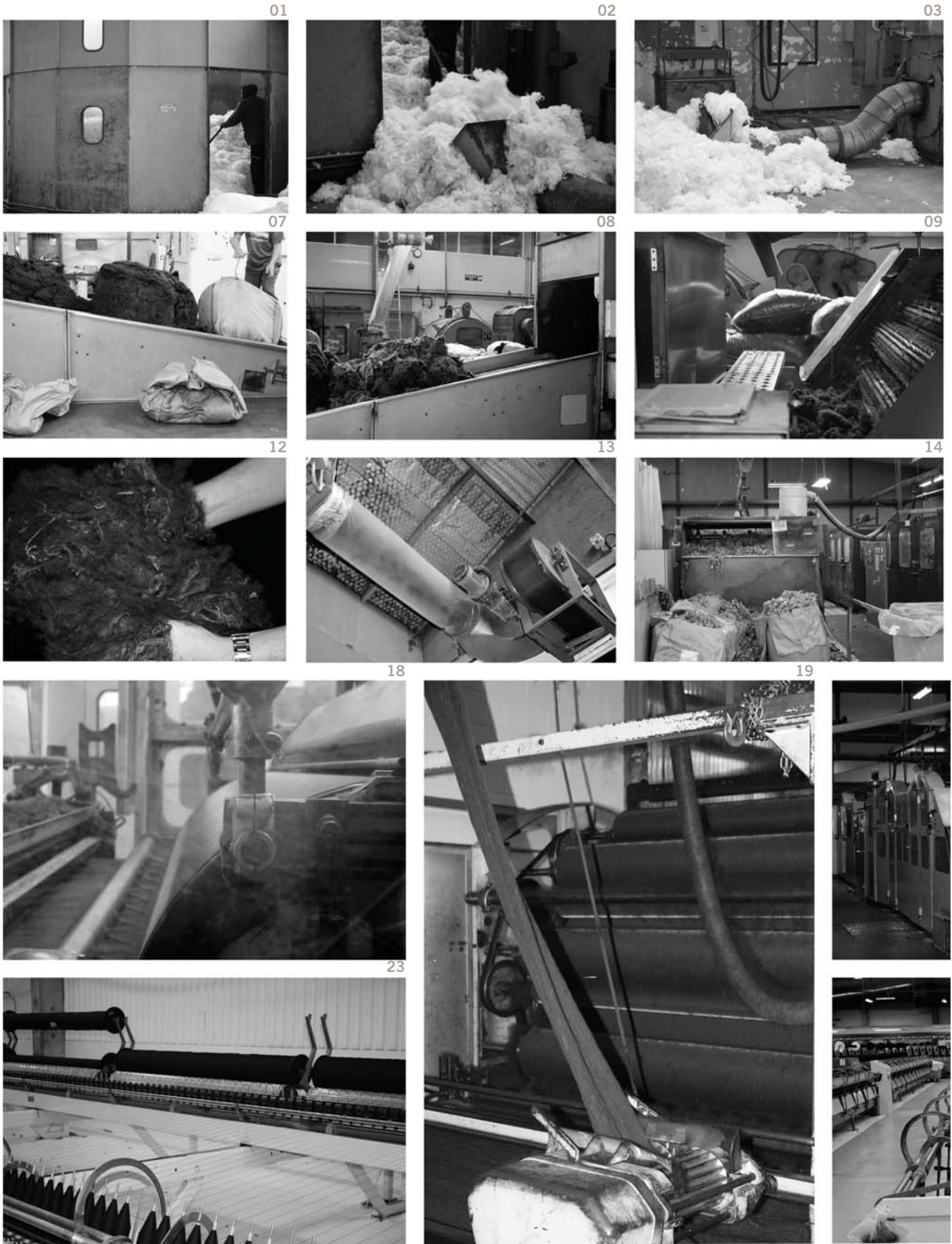
Woolyarns: 1. Oiling room 2. Oiling room 3. Oiling room 4. Fibre being transferred via 'cyclone vents' 5. The Dye house 6. The pressurized dye bath 7. Three different fibres, silk, merino, possum pre-blended / carded 8. Three different fibres, silk, merino, possum pre-blended / carded, fibre being sent to carding and blending room. 9. Sent to blending room via cyclone vents 10. Fibre being blended in blending room 11. The blended fibre 12. The blended fibre is sent to the
