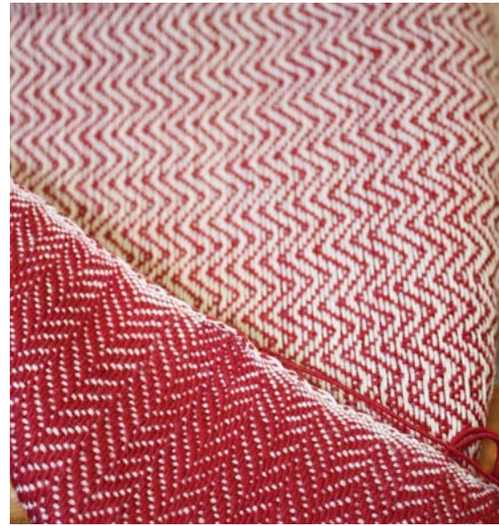
Figure 65. Hard waste yarn, woven using a twill pattern on a point draft table loom. Author's own (2012)
